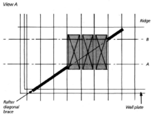
The ends of battens should be sawn square and butt jointed centrally on a rafter member. Thus, adequate bearing and nailing can be provided for each end of each batten. Butt joints in battens should be arranged so that not more than one batten in four is jointed on any one rafter member. Cantilevering or splicing of battens between rafters should not be permitted.
