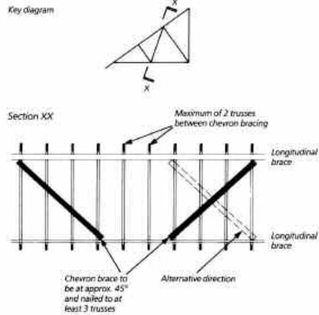
To help communications between the Trussed Rafter Designer, Building Designer, fabricator and builder the TRA have standardised on the position of the chevron bracing for the more common truss types (Figures 7.13 and 7.14).
