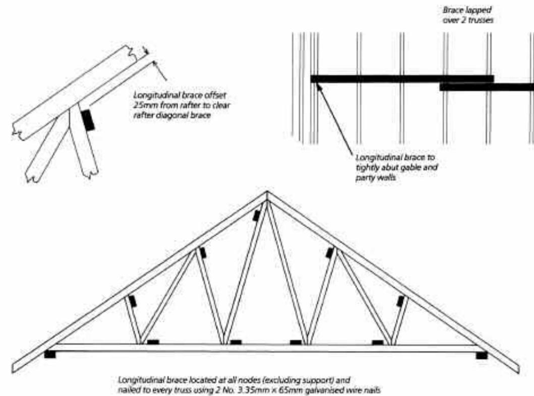
Where the truss configuration changes along a roof section, the nodes may not align. To overcome this problem, it is recommended that longitudinal binders from each roof section continue over two trusses and that both binders are located at the side of the node to minimise the distance between them (Figure 7.03).
