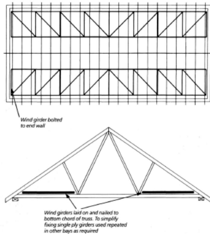
For hip ends or where the cross walls also require bracing, special details are required. To design the wind girders, the Trussed Rafter Designer needs to be given the load per metre and the amount the walls are permitted to deflect laterally, since it is often deflection rather than stress that controls the design. The typical lateral deflection permitted by Building Designers for a 4m high wall is 12mm.
