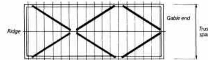
Plan of rafter diagonal bracing—monopitched roof
