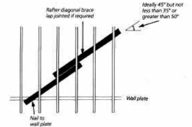
Plan of rafter diagonal bracing—narrow fronted roof
