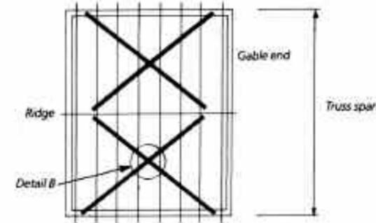
Plan of rafter diagonal bracing—wide fronted roof
