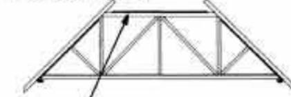
Additional diagonal bracing on horizontal top chord
