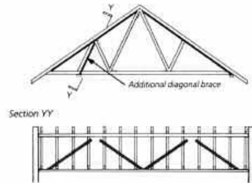
FIGURE 7.09 RAFTER DIAGONAL BRACE – ATTIC AND RAISED TIE TRUSSED RAFTERS
